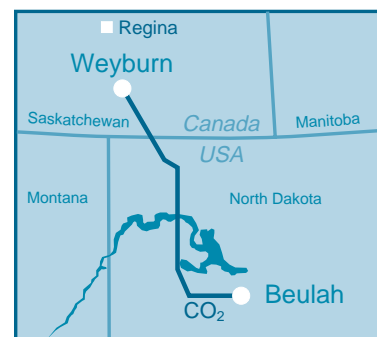
Weyburn CO 2 Flood Project For the CO 2 miscible flood, EnCana, and its partners in the Weyburn Unit, receive gas from the Dakota Gasification Company's Great Plains Synfuels Plant. This plant, located in Beulah, North Dakota, produces 160 MMcf of natural gas from coal gasification.
